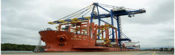
In order to optimize and strengthen the services offered by the Guayaquil Port Terminal (TPG), the Super Post Panamax Gantry crane arrived this friday, august 19, which will have a reach of up to 24 rows of containers and 48 meters of height under the spreader over the rail, making it the most modern and longest-reach crane in the country and in the region (West Coast).
